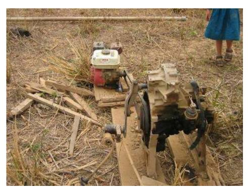
Home made adaptation for motorizing Baptist drill method. Note the 3 meter length of plastic drill stem in back ground.
