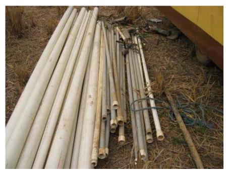
Some typical Baptist plastic PVC Drill stem and standard class 9 well casing. This drill stem is 1.25 inch schedule 40 with threaded ends with plastic couplings.
