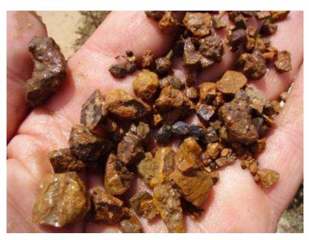
Cuttings reoved from settling pit showing what material was drilled.
